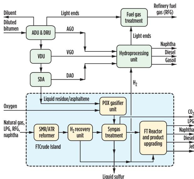
**FIG. 2.** Illustrated residue conversion concept.
